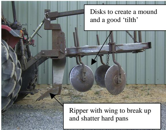
The ripper should go to a depth of 40 – 60 cm to break up any shallow hard pans. The disks create a mound of soil about 30 cm high over the rip-line.
